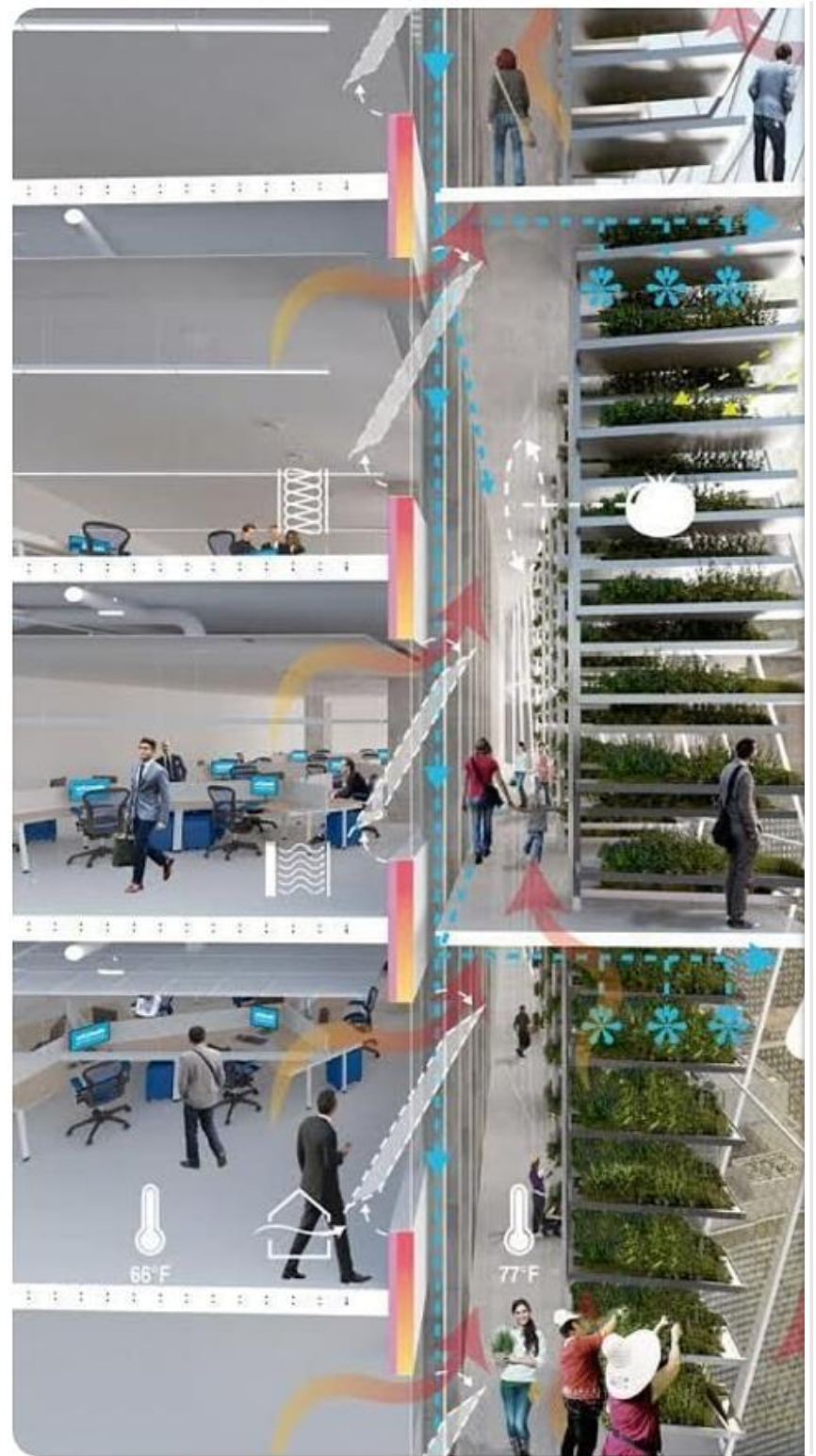
Office plan with spacious break out area around perimeter for causal meeting and amenity, which also serves as thermal buffer zone
